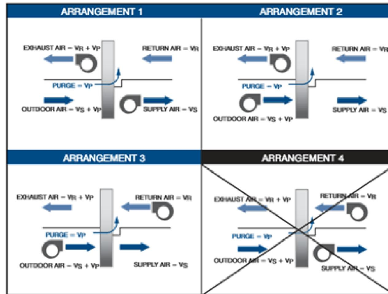
Figure 2 Fan arrangements for energy recovery exchangers
