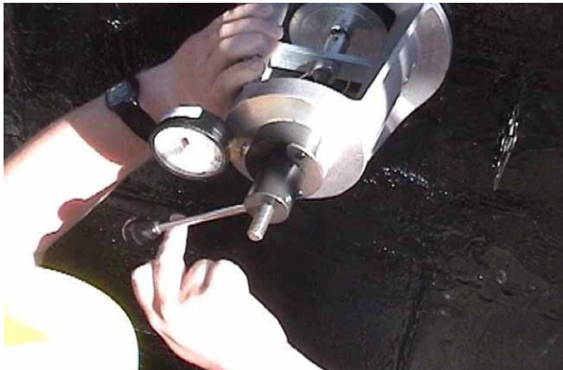
ASTM D 4541 adhesion pull testing (NIBS Guideline 3)
