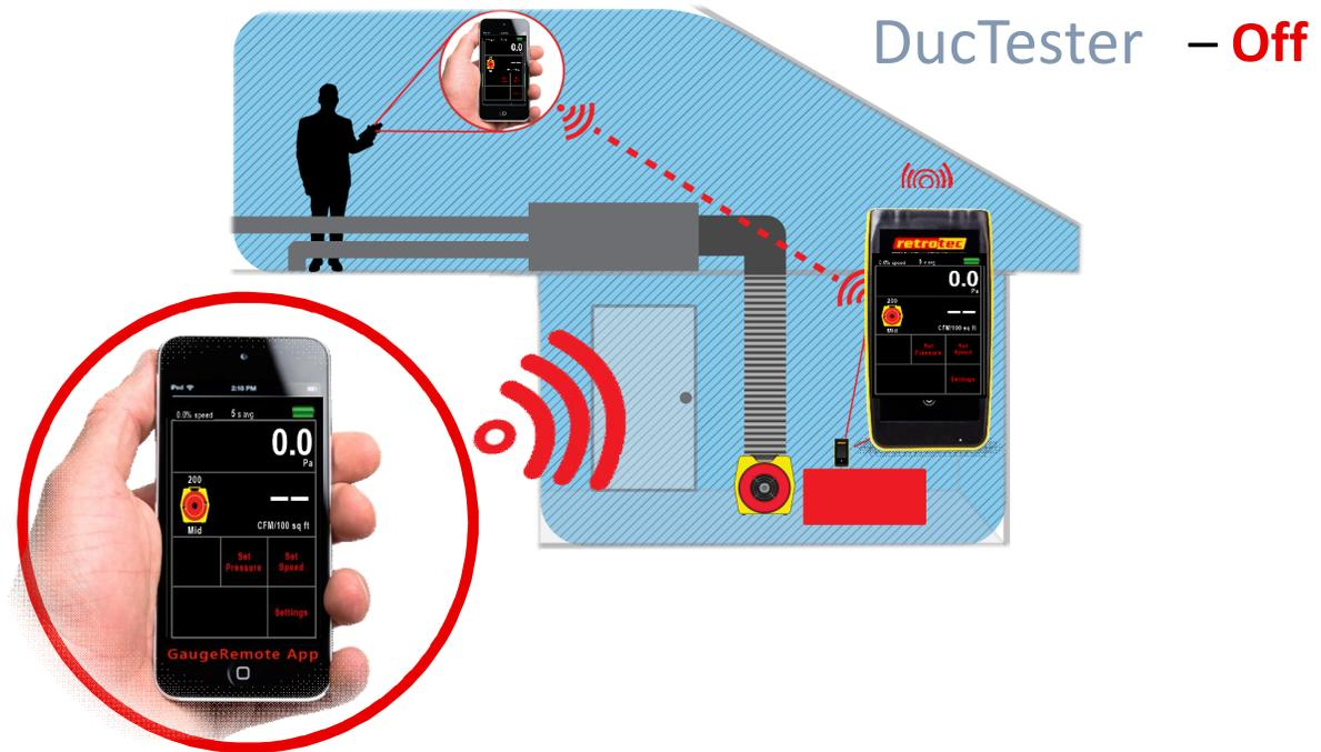
Commercial duct tester turned on and off remotely
