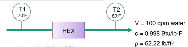
Thermocouples:  $+/- 2^{\circ}F$  (1% FS) Flowmeter: +/- 10 gpm (10% Rdg) Specific Heat uncertainty: +/- 0.0025 Btu/lb (.25%) Density uncertainty: +/- 0.16 lb/ft (.25%)
