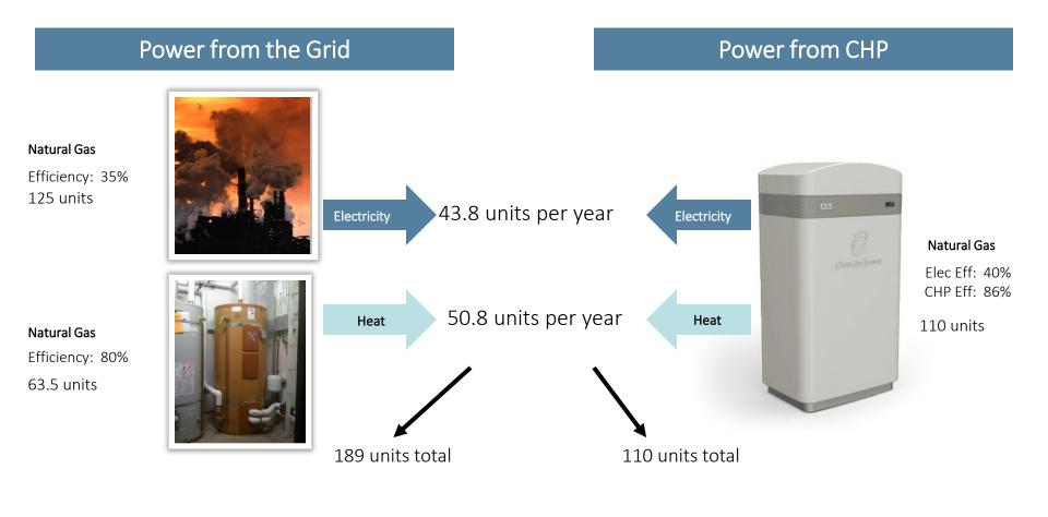
Combined Heat and Power saved **42%** reduction in fuel and CO<sub>2</sub>
