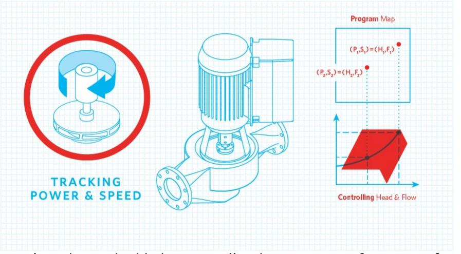
Algorithm embedded in controller that mimics performance of sensor
