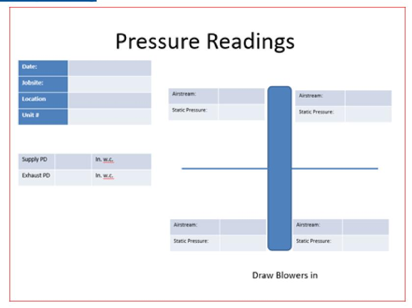
Figure 4 Field Recording Sheet for ERV Exchanger Operating Parameters
